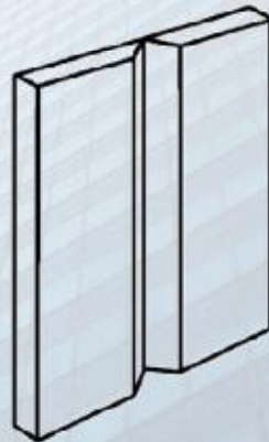
(C) VERTICAL WELDING TEST POSITION 3G
