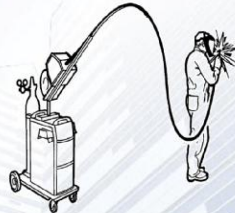
B GAS METAL-ARC WELDING WITH MAGNETIZED FLUX
